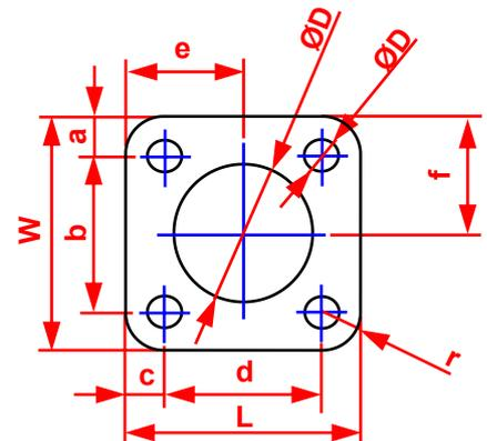
Manifold Gasket - 4 Bolt Flange
