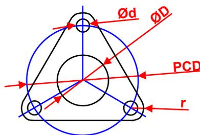
Manifold Gasket - 3 Bolt Flange
