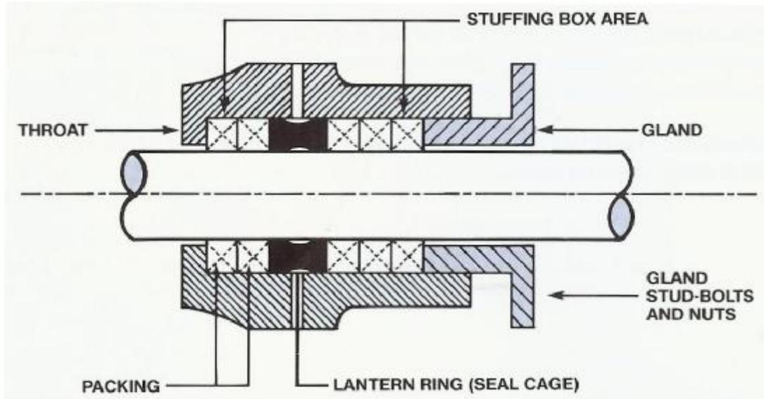
The importance of packing the pump correctly cannot be over-emphasized. Many packing failures are due to incorrect installation and maintenance of the packing. The following steps have been devised to ensure effective installation of compression packing on pumps.
